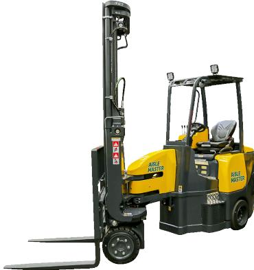
**AM 44NE – 4400lbs Capacity @ 24" Load Center – 48" Wide Chassis**
